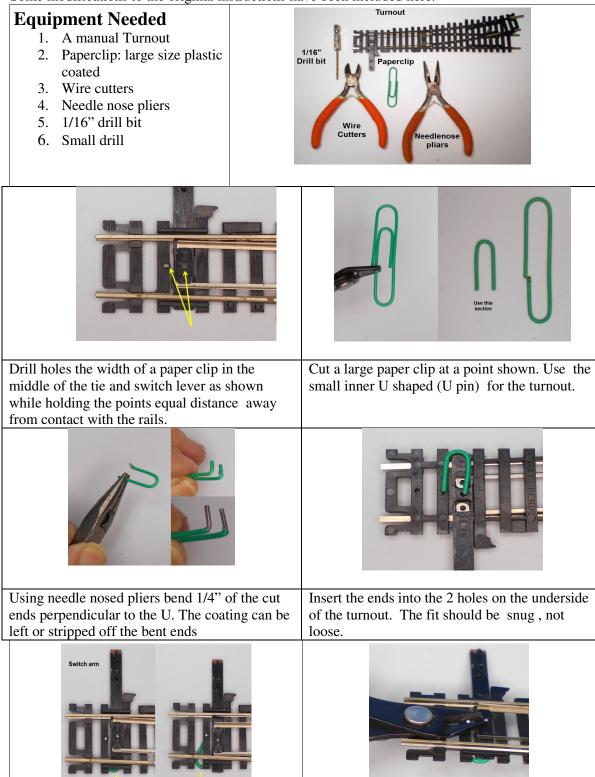
Test the switch by moving the switch arm back an forth . A small click is heard as the point secures against the track rail.
