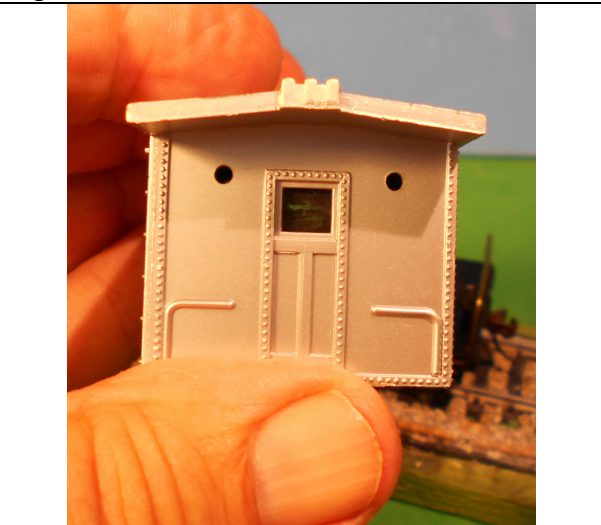
Two holes were drilled in the rear wall with a 5/64" drill bit and set approx 1 1/4" apart.
