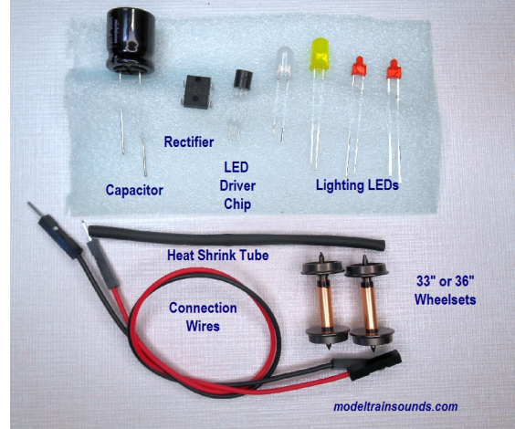
Components of the MTS Caboose LED Light kit
