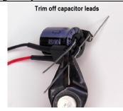
8. Trim off the excess leads extending from both Capacitor BR joints.
